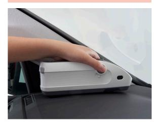
The CM-25cG's sleek, compact, lightweight body is easy to hold, and can measure even in narrow, deep-set spaces. Additionally, changeable apertures allow measurements of subjects which are small or curved.
