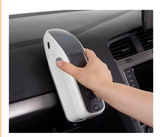
The CM-25cG greatly improves work efficiency by eliminating the need to switch between two instruments — one for color, one for gloss — for each measurement, thus reducing takt time, and providing color and gloss data from exactly the same measurement point for more accurate quality control.
